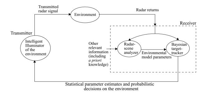
Figure 2: Block diagram of cognitive radar viewed as a closed-loop feedback system (Taken from Haykin [4])
